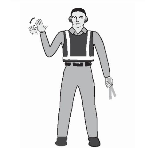
7(b) Raise hand just above shoulder height with hand closed in a fist. Ensuring eye contact with flight crew, open palm. Do not move until receipt of “thumbs up” acknowledgement from crew.
