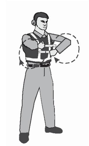
14(a) Point left arm with wand down and bring right arm from overhead vertical position to horizontal forward position, repeating right-arm movement.
