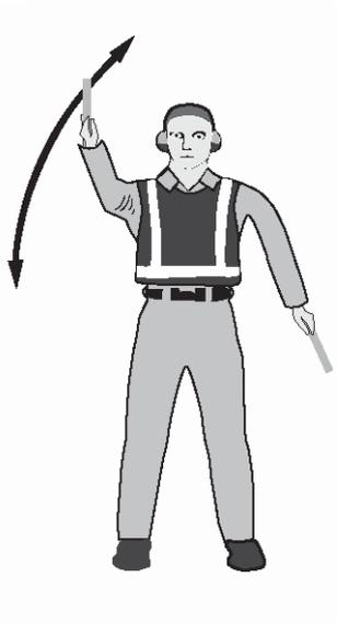
14(b) Point right arm with wand down and bring left arm from overhead vertical position to horizontal position, repeating left-arm movement.
