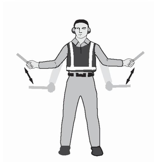
12. With arms down and wands toward ground, wave either right or left wand up and down indicating engine(s) on left or right side respectively should be slowed down.
